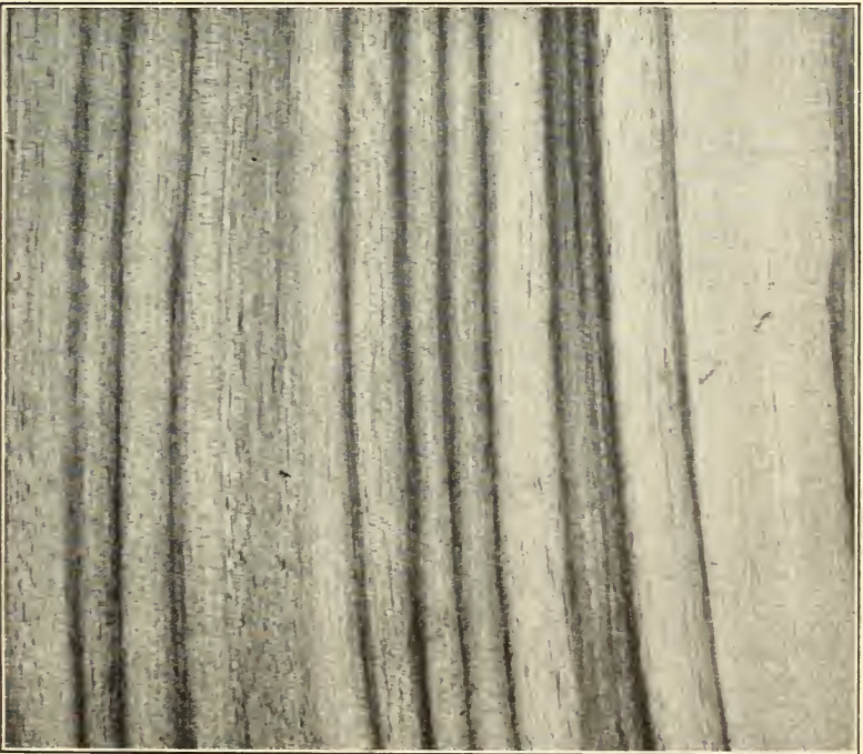
FIGS. 1 AND 2.—VENEER FROM STRAIGHT-GRAINED LOGS.
